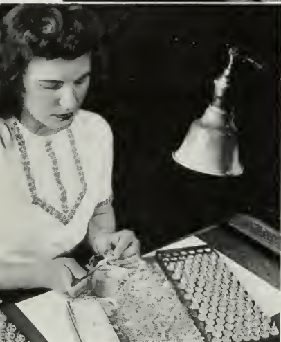
CEMENTING INSULATORS TO THE WIRE LEADS IN THE BASE OF MINIATURE TUBES TO PREVENT ELECTRON LEAKAGE.
